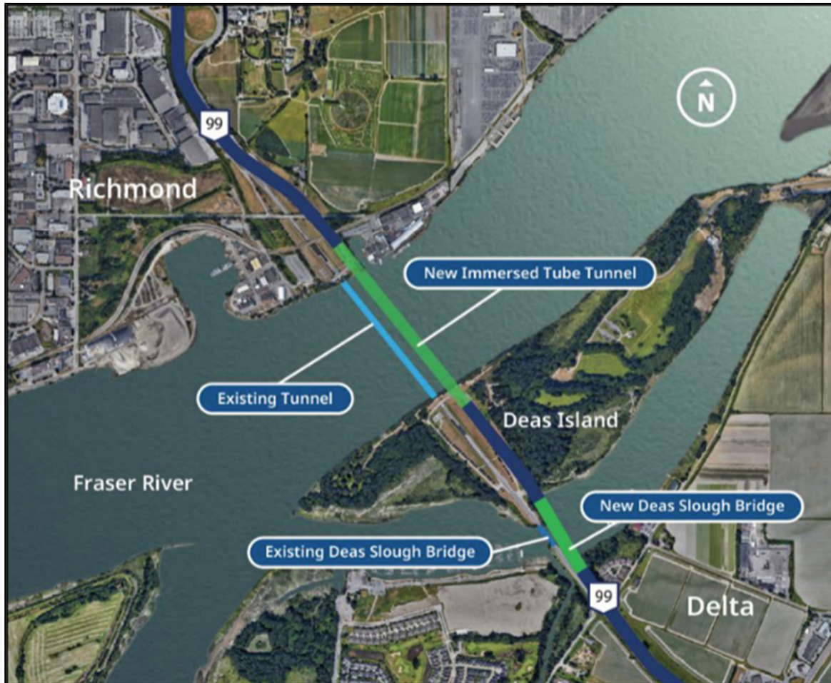
Figure 1 Fraser River Tunnel Project Overview
