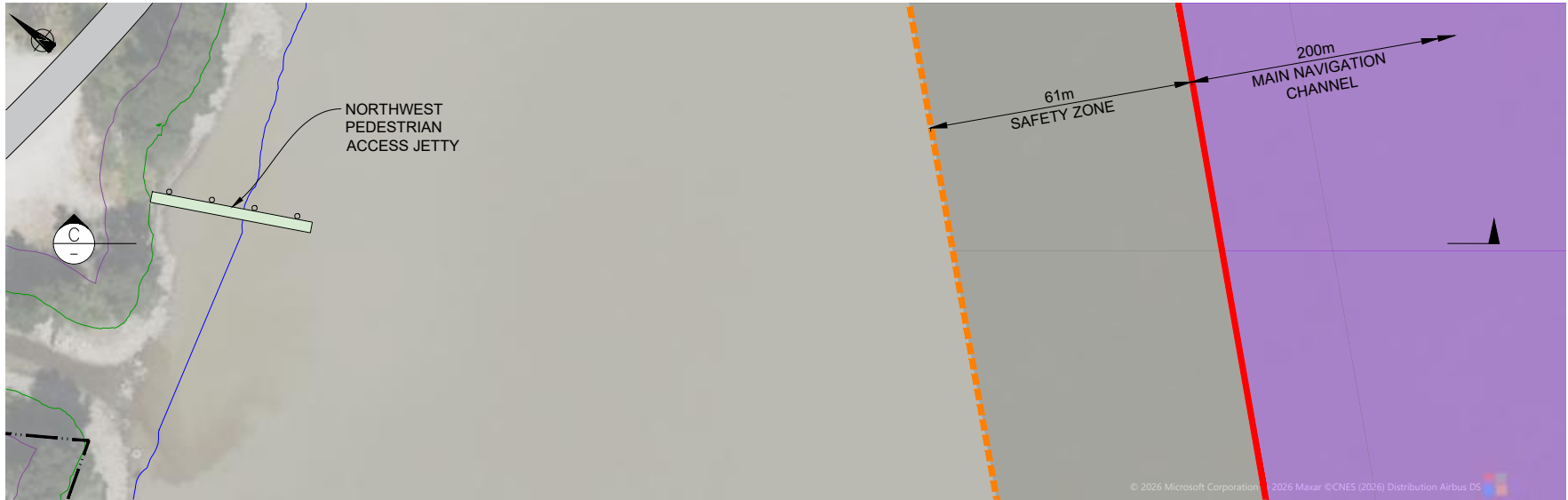
PLAN — NORTHWEST PEDESTRIAN ACCESS JETTY 1:1500
