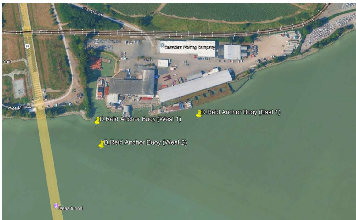
Figure 2: Derrick Barge Anchor Positions
