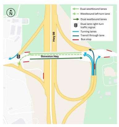
**Southbound Highway 99 off-ramp:** A second dedicated right-turn lane onto Steveston Highway westbound has been added. This new dual right-turn traffic pattern will be controlled by a traffic signal.
