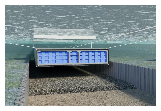
The Fraser River Tunnel Project involves immersing six tunnel elements under the Fraser River to create a new eight-lane tunnel along Highway 99. It will be located about 40 metres upstream of the existing George Massey Tunnel. When completed, the new toll-free tunnel will provide more capacity for drivers and transit users in both directions, while providing people with a walking and cycling option between Richmond and Delta.
