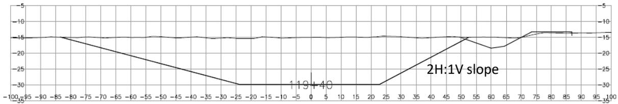
**Figure 15** Drawing of 2H:1V sloping excavation provided by Stantec (received by NHC on September 3, 2019). During an ebb (falling tide) flow is from left to right.
