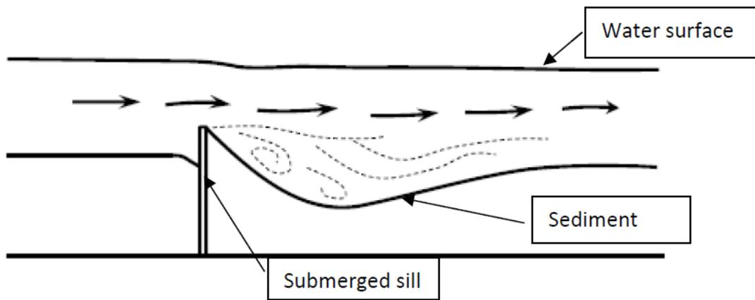
**Figure 2** Conceptual diagram of a submerged sill taken from Melville (2014) with annotations added.
