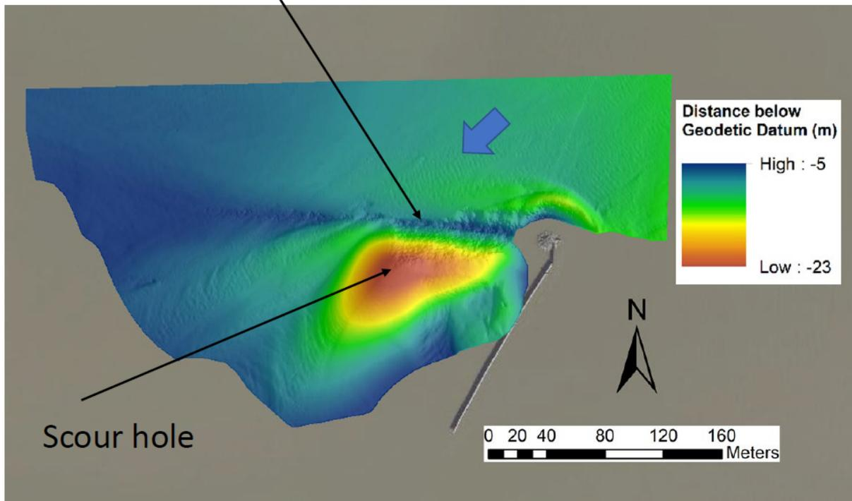
**Figure 3** Bathymetric data from Public Services and Procurement Canada at the Trifurcation Wall. During an ebb (falling tide) flow is from top to bottom.
