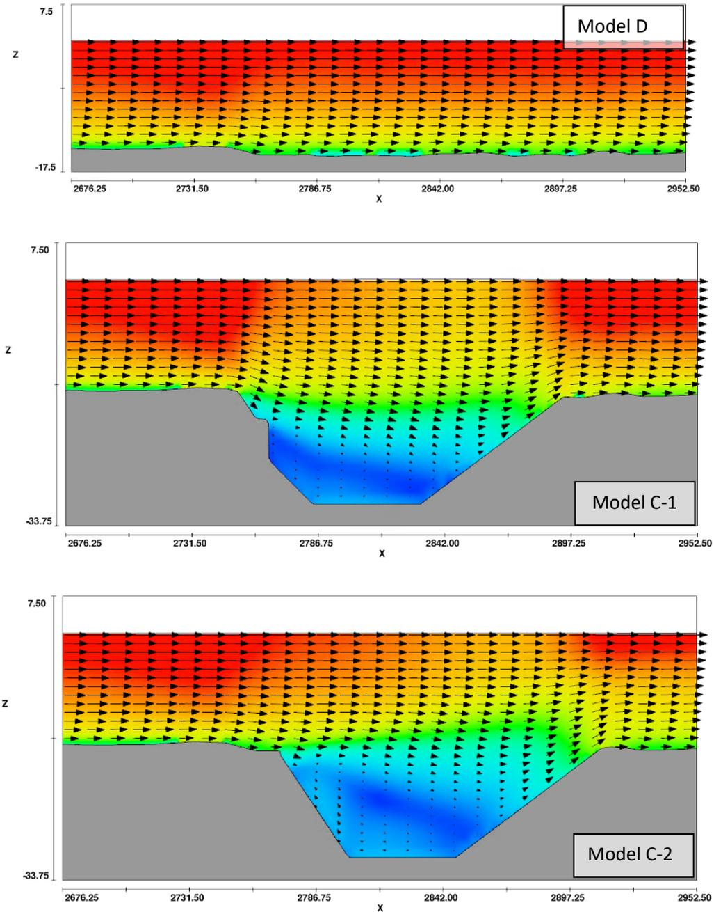
**Figure 25** Longitudinal profile in vertical plane – Velocity magnitude (m/s) simulated during the 2012 King Tide Simulations in Models C-1 and C-2. Flow is from left to right.
