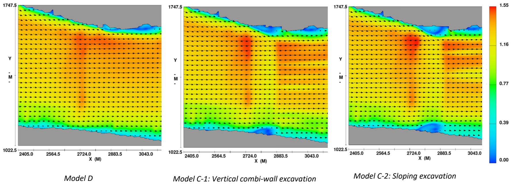
Figure 24 Plan View - Surface velocity (m/s) simulated during the 2012 King Tide Simulations in Models D (baseline), C-1 and C-2. Flow is from left to right.
