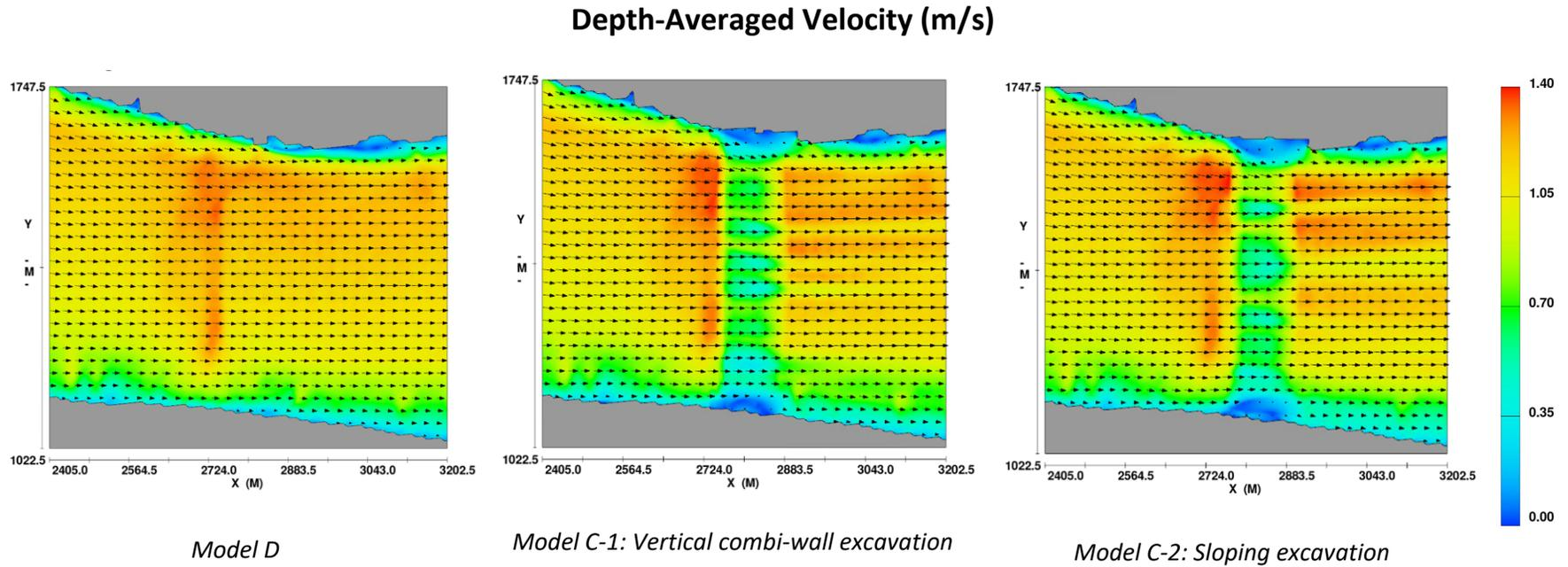
**Figure 23** Plan View - Depth-averaged velocity (m/s) simulated during the 2012 King Tide Simulations in Models D (baseline), C-1 and C-2. Flow is from left to right.
