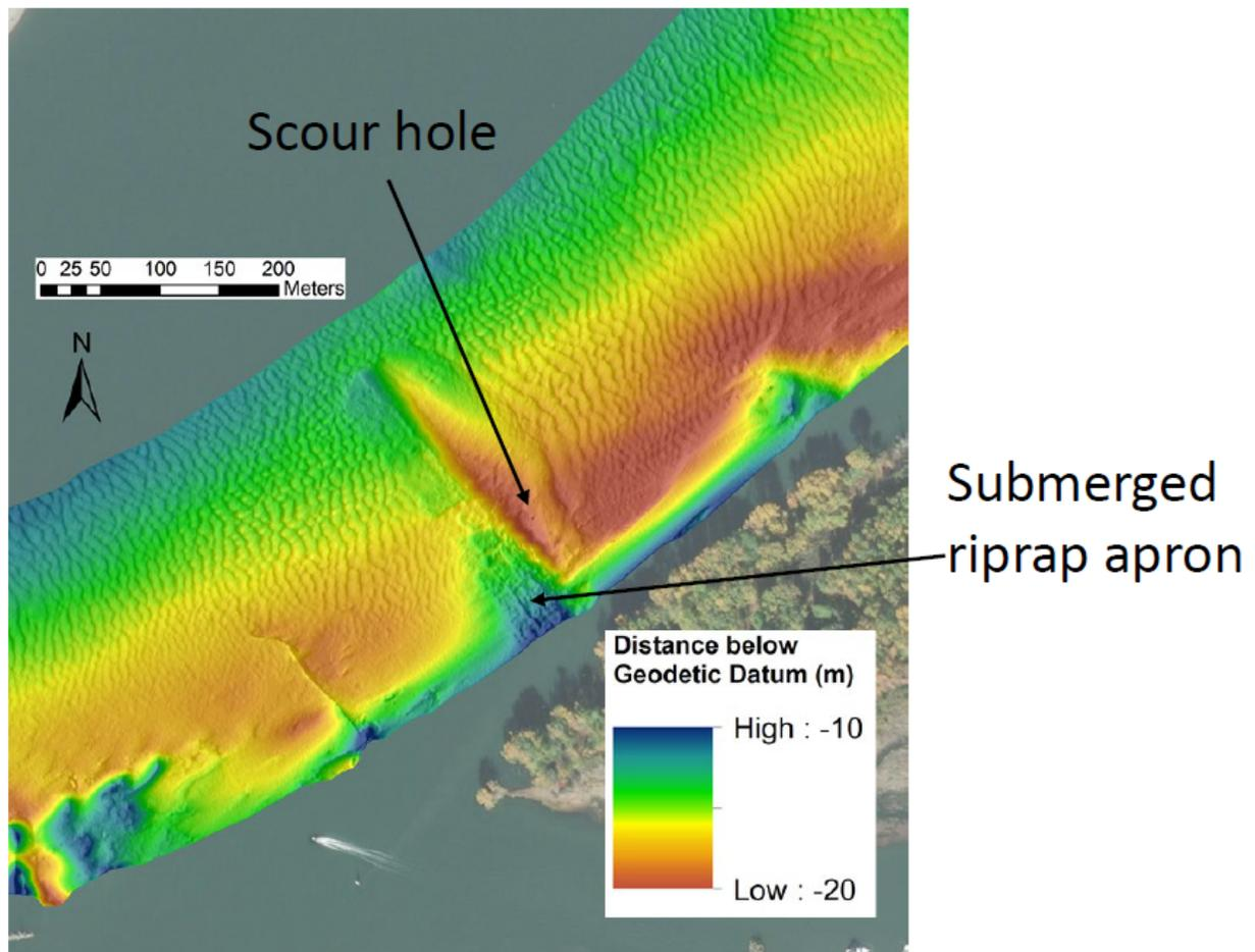
**Figure 5** Bathymetric data from Public Services and Procurement Canada at the Lulu Island-Delta Water Main. During an ebb (falling tide) flow is from top right to bottom left.
